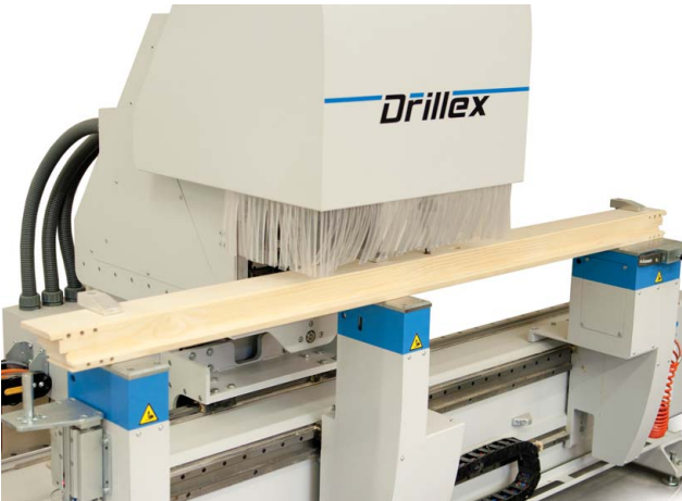
Exchangeable drilling heads for handle and window hinges
