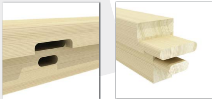
Mortised slots with rounded tenons
