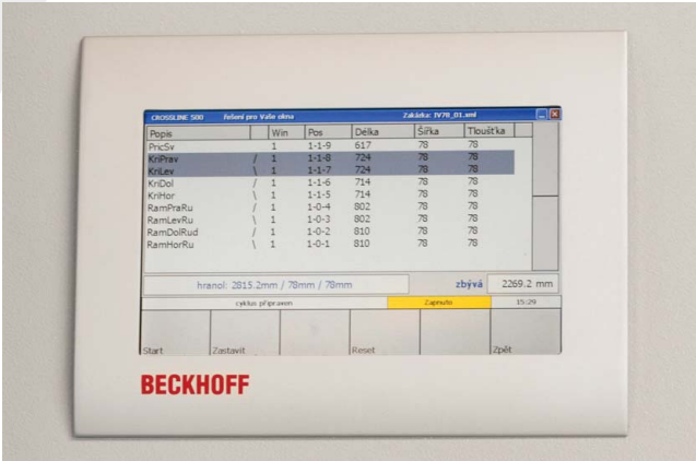
industrial computer with 7" touch screen for manual control or with data from WinCreator.
