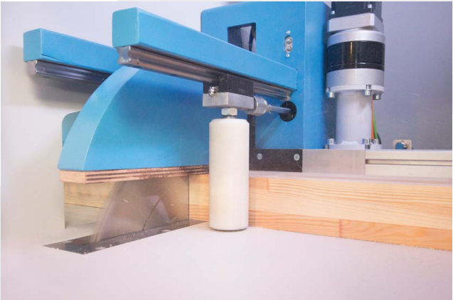
side and top clamp for precise cut
